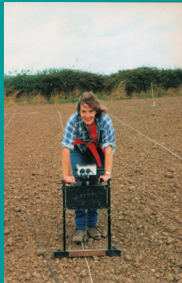
Sue Gaffney with RM4, P1 and current booster on metal plate
