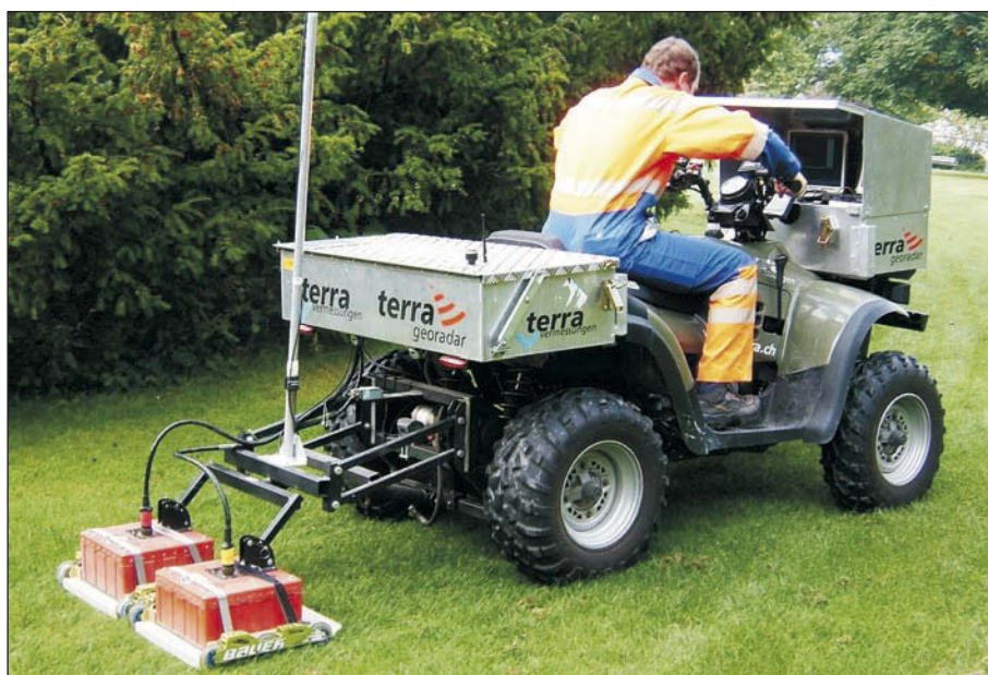
Fig. 1. Quad with two GPR antennas and prism for the real-time positioning system, used to survey the areas.
