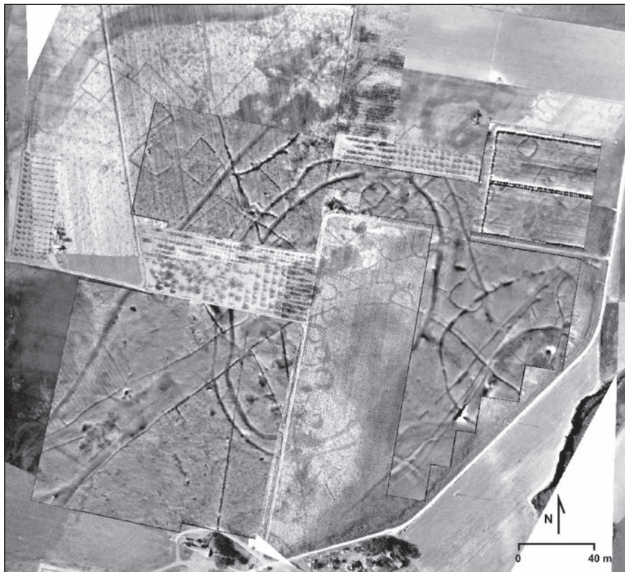
Fig. 2. Processed magnetograms displayed in 256 grey tone (-25 white, +25 black) nT, and overlapped to the orthorectified aerial photographs. The magnetic and aerial data appear highly correlated. The good readability of the signals was achieved after all the processing procedures and by applying DIP techniques.
