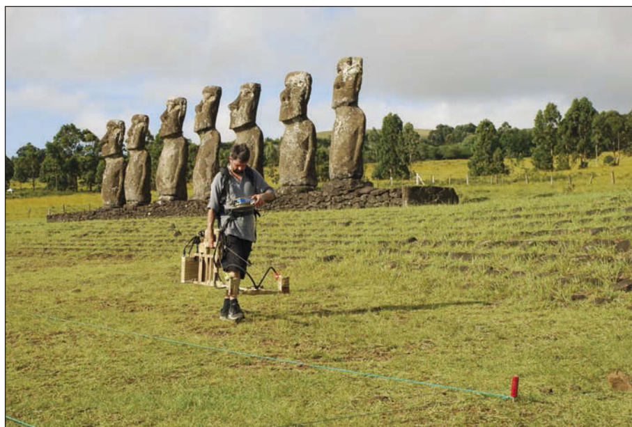
Fig. 1. Ahu Akivi. One of the authors prospecting in front of the Ahu Akivi site with the optical pumped caesium magnetometer.
