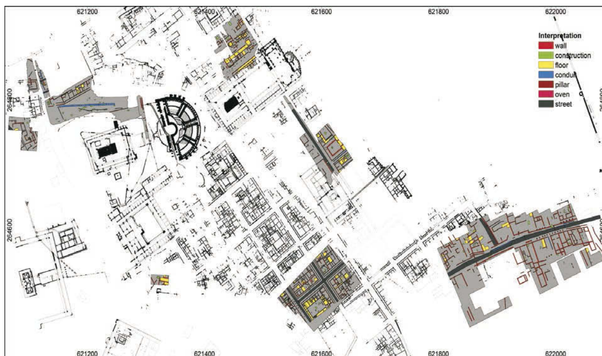
Fig. 2. Plan of the Roman site Augusta Raurica with the interpretations of the ground-penetrating radar data in colour and the already excavated structures in black.
