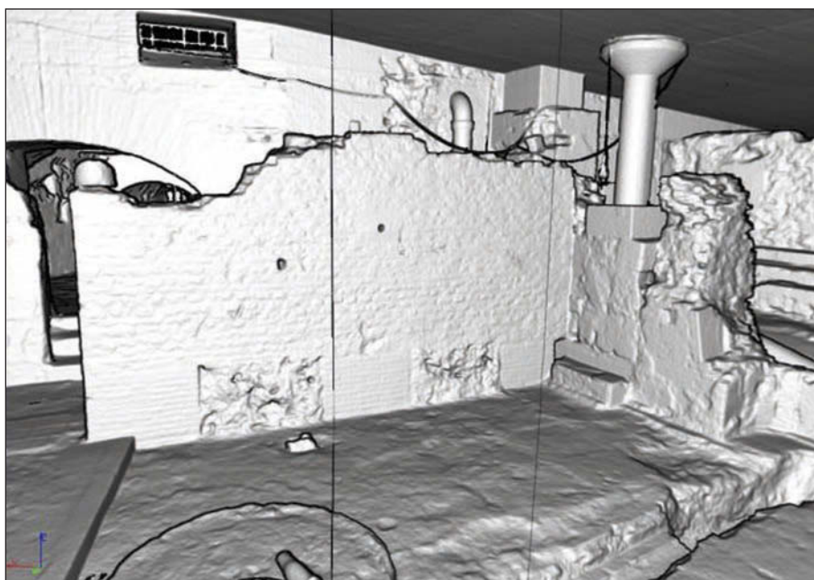
Fig. 2. Laser scanner survey. 3D model of the Nymphaeum complex.
