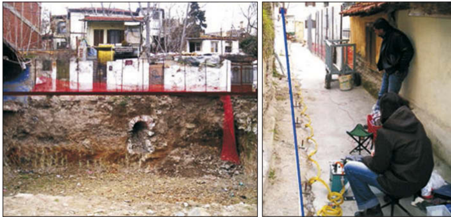
Fig. 2. The left part shows the Roman pipe being cut when the trench was opened for the foundations of a modern building. The line of the flat base electrodes used along with the multicore cable. The arrows depict the tomographic transect.
