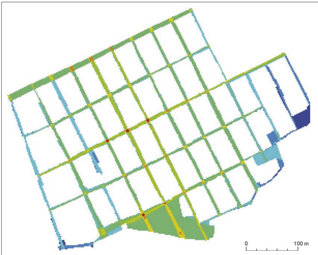
Fig. 3. Visibility graph analysis of the street network: the irregularities of the Hippodamian are highlighted. The visualization of the "integration" parameter (minimum blue/maximum red) shows a slightly different hierarchical organization of the streets than with the axial map.
