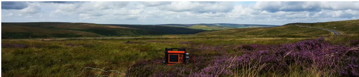
Figure 3: ABEM Terraloc Pro seismograph mapping upland peat deposits.
