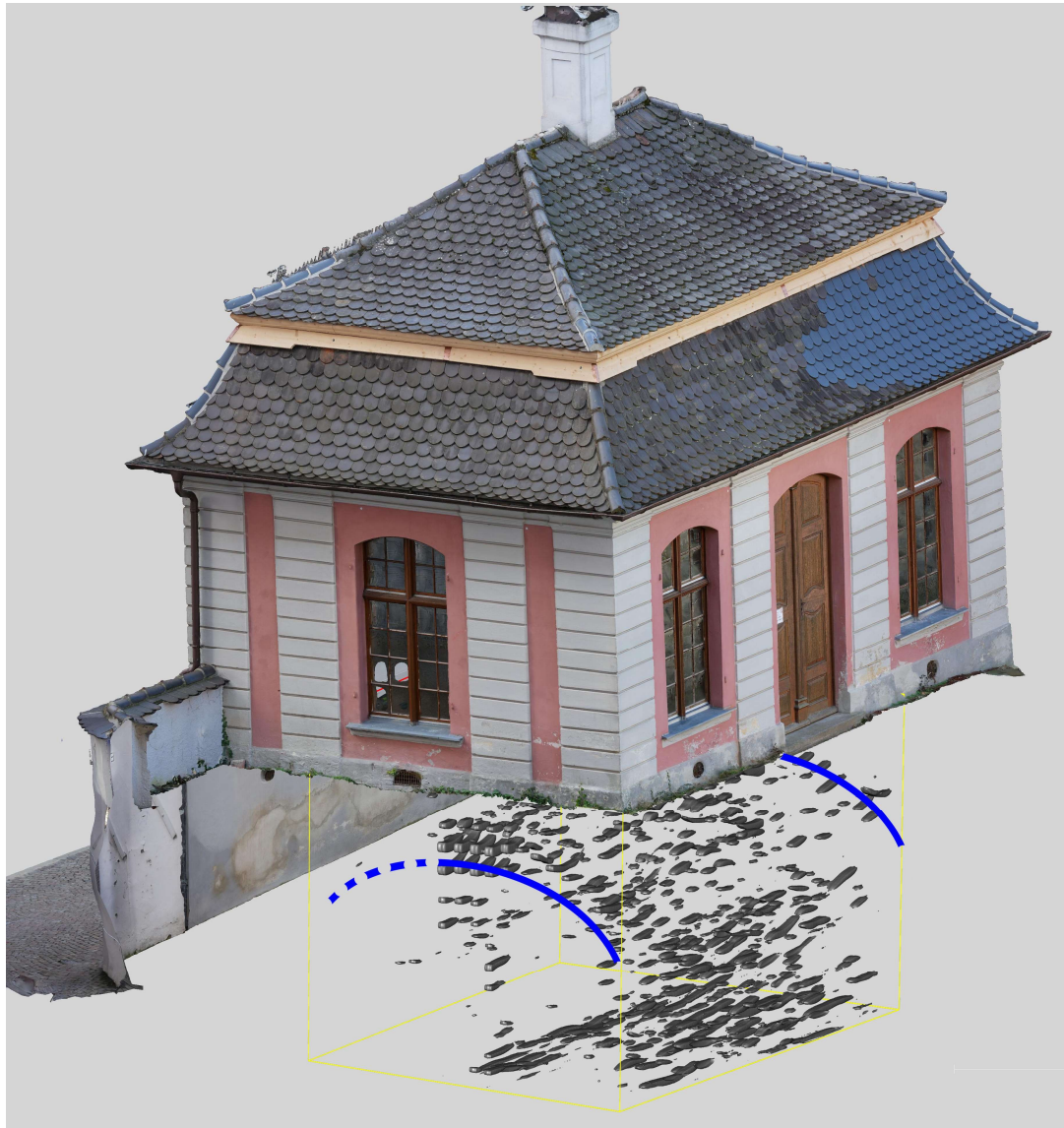
Figure 4: Photogrammetric 3D-model of the Baroque garden pavilion with the modelled GPR results of the barrel vault displayed underneath. The blue lines illustrate the position of the bricked vault.
