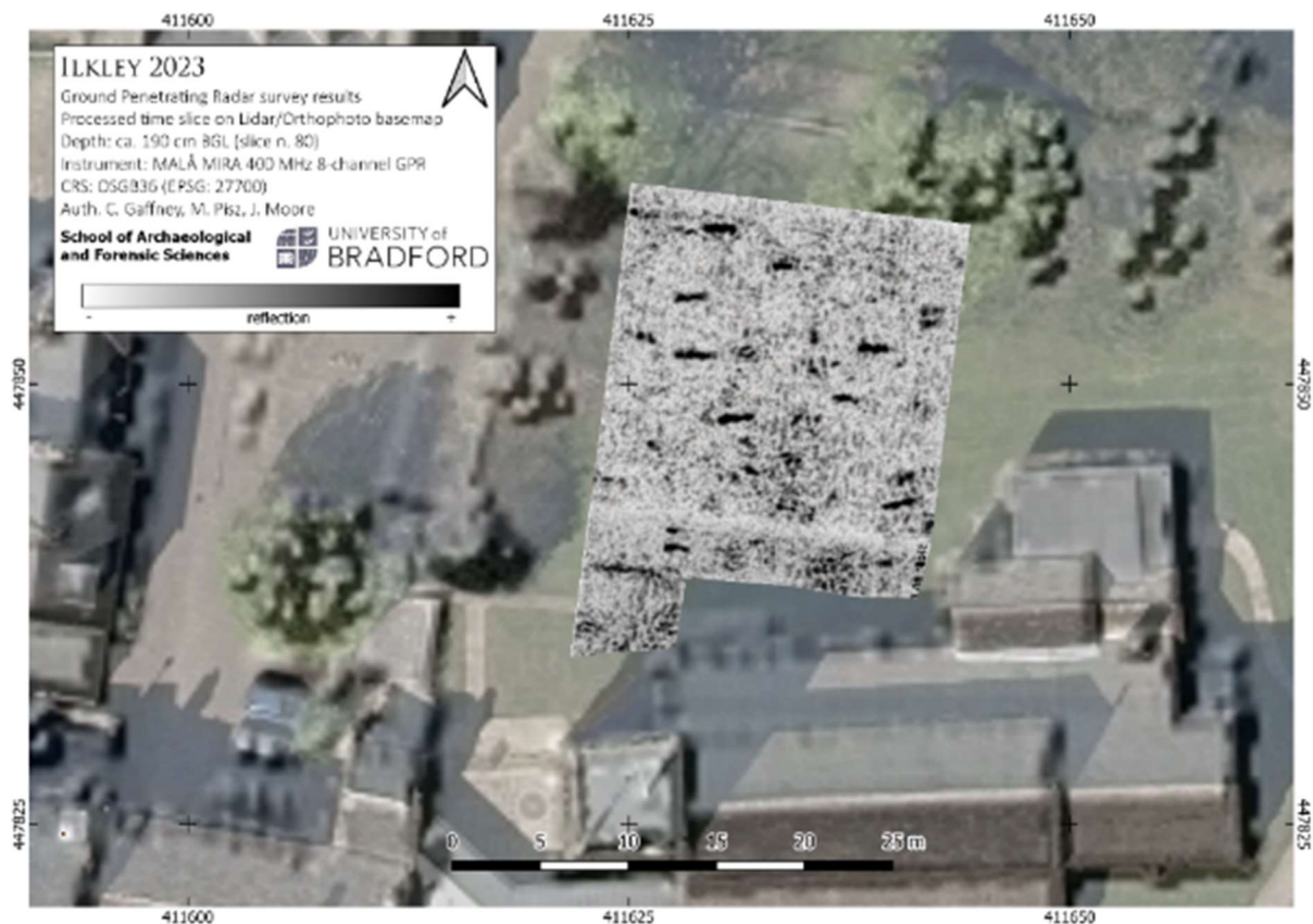
Figure 2 – 3D GPR Mala MiniMIRA data processed using the SubGeo WAVE GPR software.
