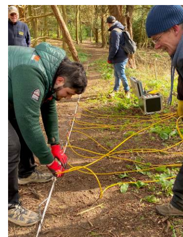
Figure 2: Electrical Resistivity Imaging (ERI) data over a WW2 OB in Wiltshire, UK
