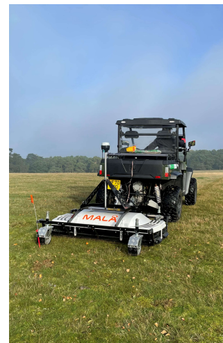
Figure 1: MALÅ MIRA HDR multichannel 3D GPR array
