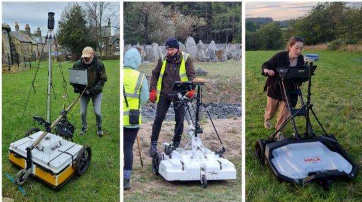
Figure 1 – Three different 3D GPR systems (from left to right): Malå MiniMIRA, ImpulseRadar Raptor 45 and Malå MIRA Compact
